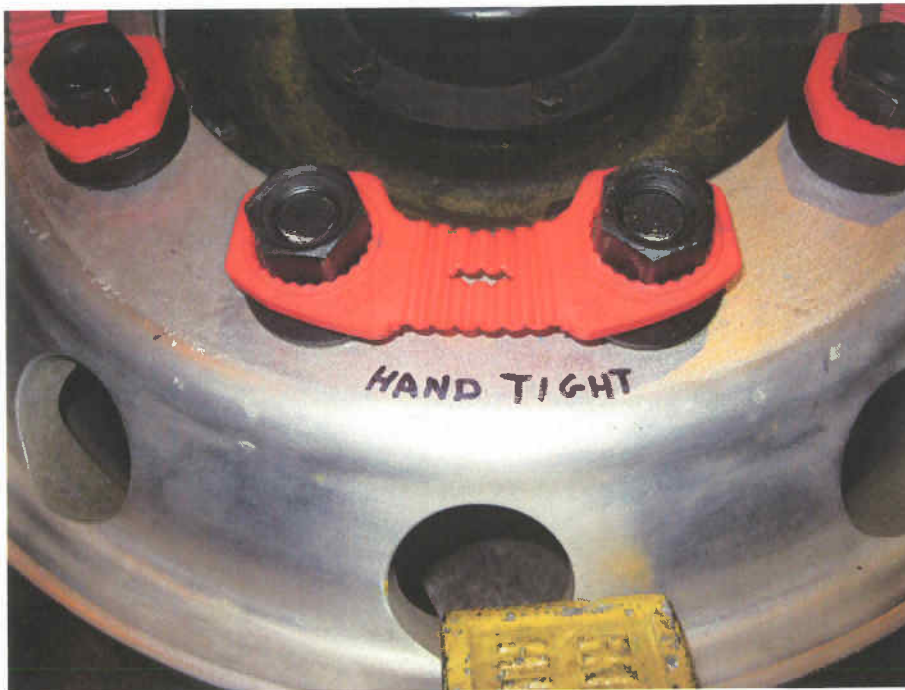
Figure 8 : Sample 10-03-C0152-6 installed on hand tight nuts
