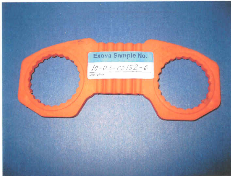
Figure 18 : Sample 10-03-C0152-6 after test (left nut tightened with air gun)
