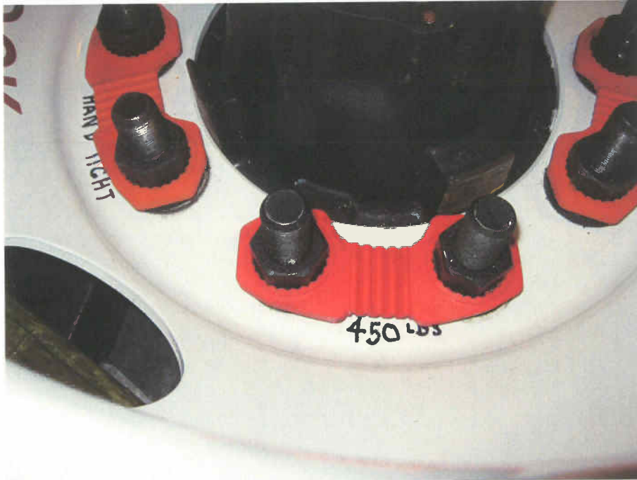
Figure 7 : Sample 10-03-C0152-5 installed on 450 ft-lb torque nuts
