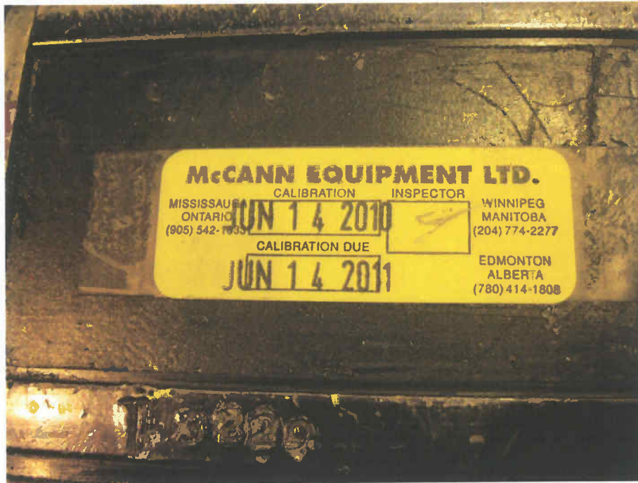
Figure 1A : Photo of air gun calibration sticker
