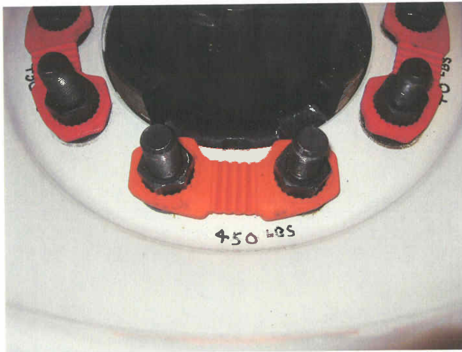
Figure 6 : Sample 10-03-C0152-4 installed on 450 ft-lb torque nuts
