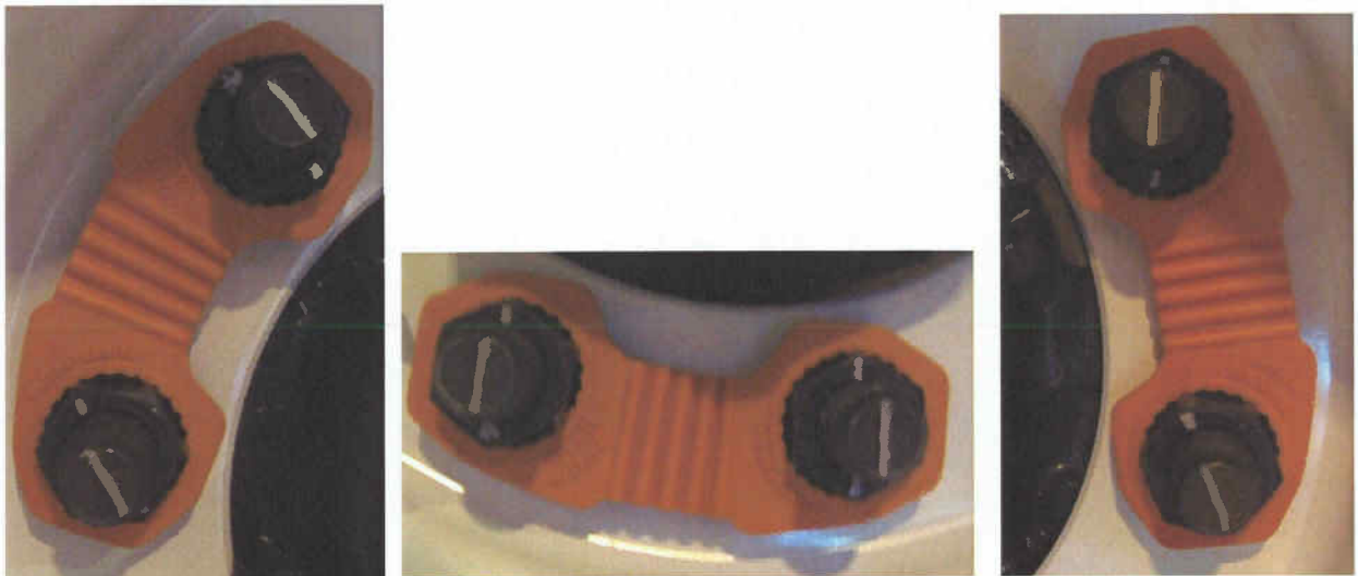
Figure 2A: Photos of Zafety Lug Lock prior to vibration test at 25 °C
