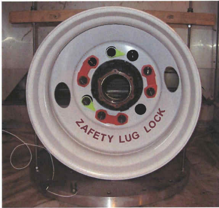
Figure 1A: Vertical vibration test set-up at 25 °C
