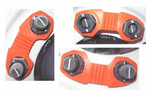
Figure 5A: Photos of Zafety Lug lock after vibration test at -40 °C
