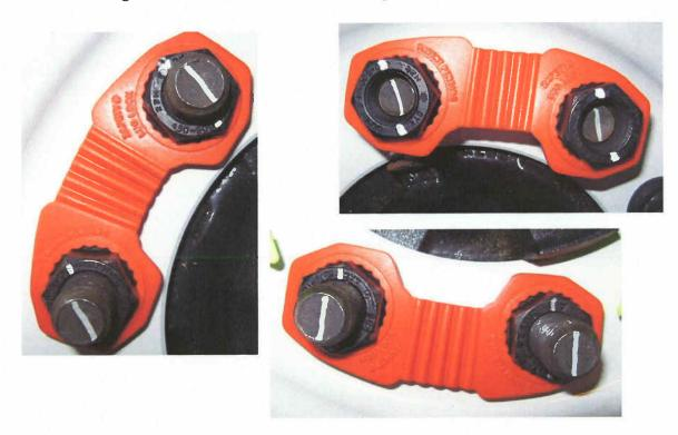
Figure 4A: Photos of Zafety Lug lock prior to vibration test at  $55\,^{\circ}\mathrm{C}$
