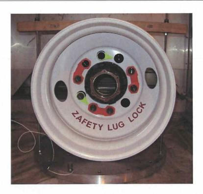
Figure 1A: Vertical vibration test set-up at 25 °C
