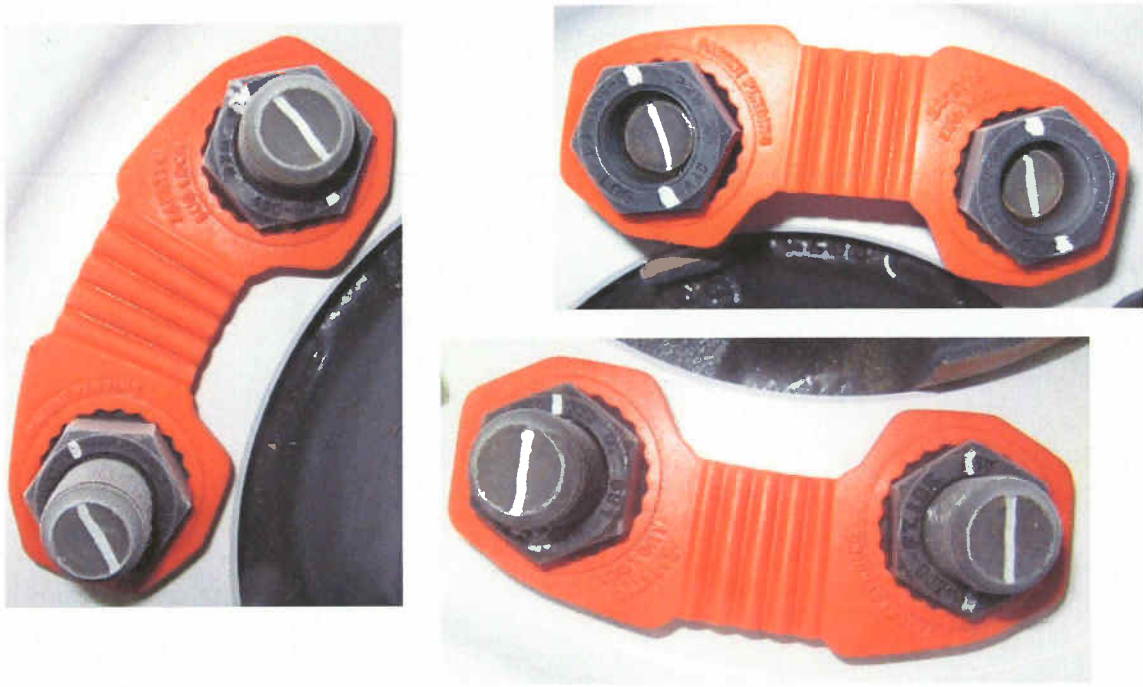
Figure 5A: Photos of Zafety Lug lock after vibration test at -40 °C
