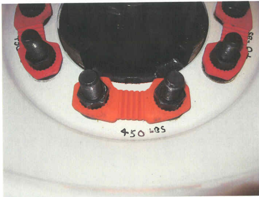
Figure 6 : Sample 10-03-C0152-4 installed on 450 ft-lb torque nuts
