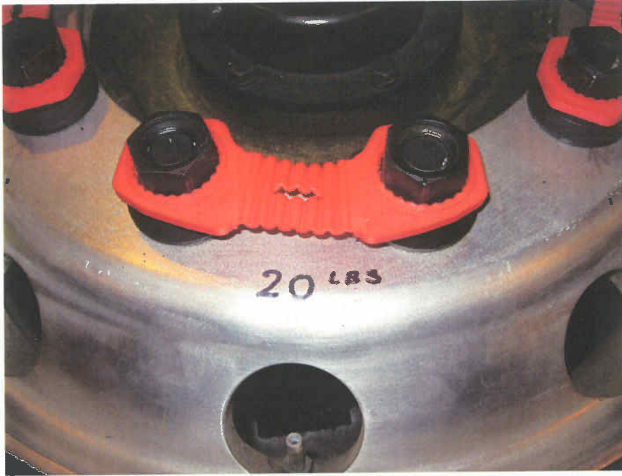
Figure 9 : Sample 10-03-C0152-7 installed on 20 ft-lb torque nuts
