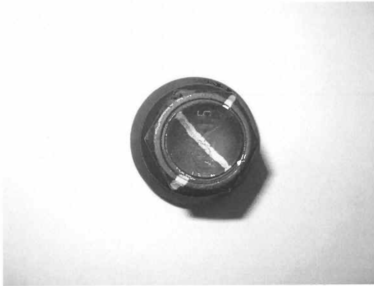
Figure 7A Wheel nut with installed cap washer
