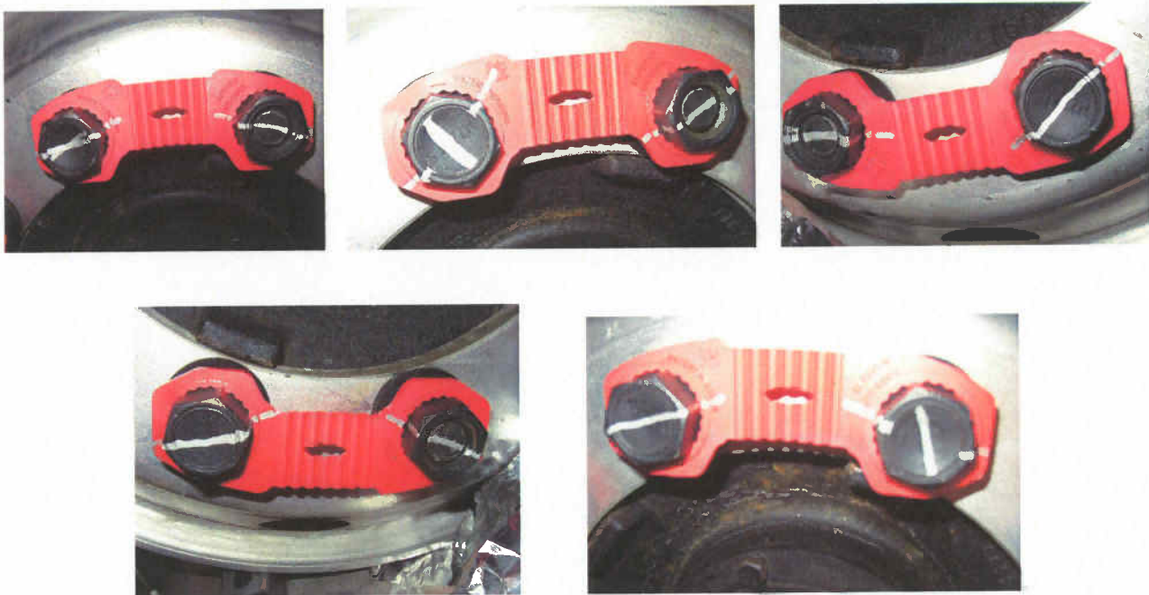
Figure 4A The various lug nuts and Safety Lug Lock units, indicating the position of the lug nuts after testing at 150°C
