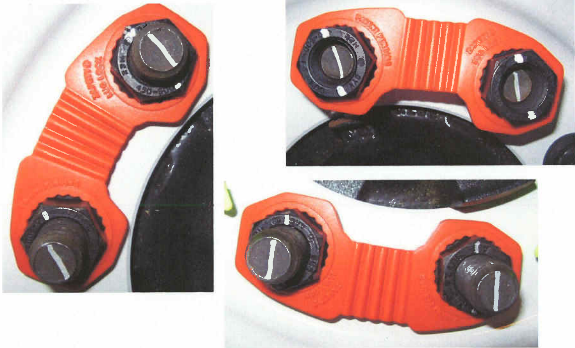
Figure 4A: Photos of Zafety Lug lock prior to vibration test at 55 °C
