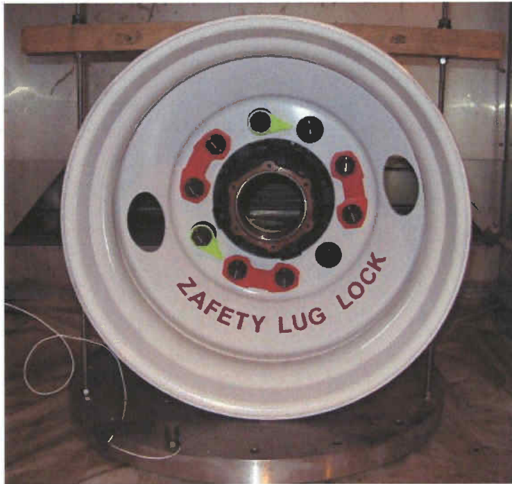
Figure 1A: Vertical vibration test set-up at 25 °C
